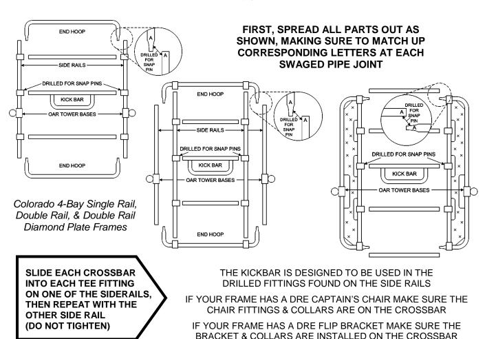
FINALLY, INSTALL ONE END HOOP & PIN BOTH JOINTS INTO PLACE / REPEAT ON OTHER SIDE
